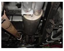
SLIDE MUFFLER #C ONTO HEADPIPES 1-1/2" TO 2". OUTLETS SHOULD BE AT THE BOTTOM. USE A JACK STAND TO SUPPORT MUFFLER AND ATTACH TO HEADPIPES WITH CALMP #G.
