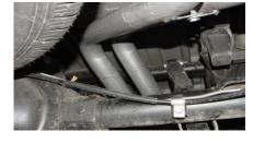
SLIDE PASSENGER SIDE TAILPIPE #E INTO MUFFLER 1-1/2" TO 2". USE CLAMP #I TO SECURE TAILPIPE TO MUFFLER. DO NOT TIGHTEN.
