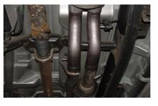
SLIDE PASSENGER SIDE HEADPIPE #A ONTO STOCK HEADPIPE. INSERT WELDED HANGER INTO RUBBER GROMMET. NEXT INSTALL DRIVERS SIDE HEADPIPE #B ONTO STOCK HEADPIPE, USE CLAMP #H TO SECURE BOTH HEADPIPES. DO NOT TIGHTEN.
