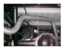
INSTALL DRIVER SIDE TAILPIPE #D INTO MUFFLER 1-1/2" TO 2" AND USE CLAMP #G TO SECURE THE MUFFLER. DO NOT TIGHTEN. USE CLAMP #G TO HOLD PIPE UP TO THE HANGER #F.
