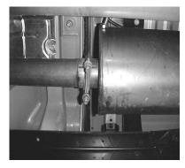
DO NOT REMOVE THE EXTENSION PIPE BETWEEN THE MUFFLER AND THE CONVERTER.
