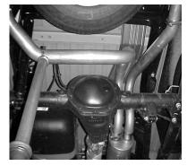
INSTALL PASSENGER SIDE OVERAXLE PIPE #D AND ATTACH TO MUFFLER USING CLAMP # F. INSERT HANGER INTO RUBBER.
