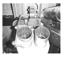
MEASURE 22" FROM THE REAROF THE FRAME. INSTALL TAILPIPE HANGER # G USING HARDWARE PROVIDED.
