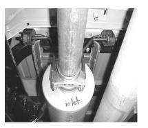
INSTALL MUFFLER ONTO STOCK HEADPIPE AND ATTACH WITH FRONT MUFFLER HANGER # I AND INSERT INTO RUBBER GROMMETS. ALIGN NOTCH ON GIBSON MUFFLER TO STOCK ALIGNMENT PIN ON FACTORY HEADPIPE. MUFFLER INLET IS TOWARDS THE CONVERTER .USE A JACK STAND TO SUPPORT THE MUFFLER.
