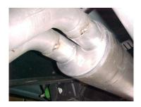
Install muffler# C onto head pipes 1-1/2" to 2" with the louvers facing towards the converter. Use a jack stand to support the muffler. Use clamps #G to the secure the muffler to the head pipes. Do not tighten
