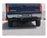
Install exit pipes #F. Use clamps #H to secure exit pipes to tailpipes. These clamps also attach to the metal hangers. Rotate to adjust for clamping. Now go back and tighten up all clamps, nuts, and bolts.
