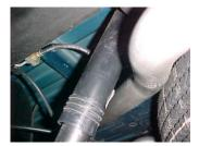
Install driverside overaxle tailpipe #E into muffler  $1 \frac{1}{2}$ " to 2". Support end of tailpipe with jack stand and attach to hanger #H.
