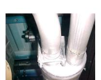
Next, install rear muffler hanger #H onto drivers side muffler outlet and insert hanger into rubber grommet. Do not tighten.
