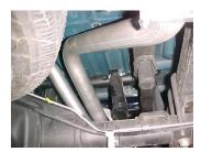
Install passenger side overaxle tailpipe #D into muffler 1  $\frac{1}{2}$ " to 2". Secure with clamp #I. Do not tighten.
