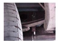
Install metal hangers # I Into holes located approximately 22" from the rear of the frame. Metal hangers are mounted on the outside of the frame. Use bolt kit #K. The bolt and the washer will go into the 3<sup>rd</sup> hole from the top of the hanger.
