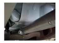
Install the passenger side tailpipe # C into the muffler at least 1-1/2" to 2". Use clamp # H to secure pipe to muffler. Do not tighten. The tailpipes both will lean towards the driver side for clearance.
