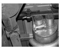
INSTALL MUFFLER #B ONTO HEADPIPE AT LEAST 1  $\frac{1}{2}$ " TO 2". USE CLAMP #F TO SECURE MUFFLER TO HEADPIPE. DO NOT TIGHTEN. USE A JACK STAND TO SUPPORT THE MUFFLER. OUTLETS SHOULD BE AT THE TOP. INSTALL HANGER #I ONTO DRIVERSIDE MUFFLER OUTLET AND INSERT WELDED HANGER INTO GROMMET. DO NOT TIGHTEN.
