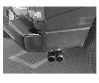
INSTALL THE STAINLESS TIPS. NOW GO BACK AND TIGHTEN ALL CLAMPS, NUTS AND BOLTS STARTING FROM THE FRONT AND WORKING BACK. TO CLEAN TIPS USE A SCOTCH BRITE PAD AND ANY STAINLESS CLEANER.
