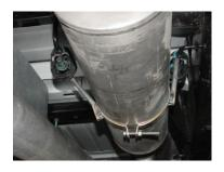
INSTALL MUFFLER #B ONTO HEADPIPE 1-1/2" TO 2". USE CLAMP #G TO SECURE THE MUFFLER TO THE HEADPIPE. DO NOT TIGHTEN. SLIDE BAND CLAMP #H ONTO THE MUFFLER AND INSERT THE WELDED HANGERS INTO THE RUBBER GROMMETS. ATTACH WITH BOLT KIT #J.
