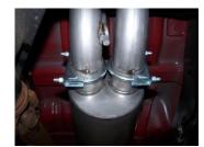
6. Slide the passenger side tailpipe #D into muffler 1.5-2". Insert welded hanger into rubber grommet. Use clamp #F to secure tailpipe to muffler. Do not tighten.
