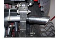
axle tailpipe #E into muffler 1.5-2". Use clamp #G to secure. DO NOT TIGHTEN. Insert welded hanger into rubber grommet.
