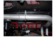
6. Install driver side exit pipe #D onto over axle tailpipe. Use clamp #G to secure. DO NOT TIGHTEN. Insert welded hanger into rubber grommet.
