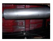
4. Install muffler #B onto headpipe 11/2"-2" with the louvers facing towards the converter. Use a jack stand to support the muffler. Use clamp #G to secure the muffler to the headpipe. DO NOT TIGHTEN.
