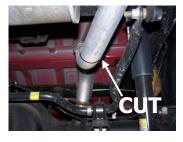
3. Install headpipe #A onto vour existing stock flange using bolt kit #H to secure flange. DO NOT TIGHTEN. Insert welded hanger into rubber grommet.
