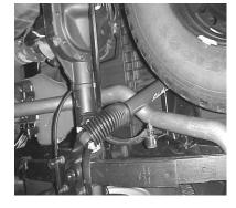
INSERT WELDED HANGER INTO THE RUBBER GROMMET.
