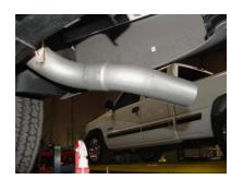
INSTALL YOUR EXITPIPE #D AND USE CLAMP #H TO SECURE THE PIPES TOGETHER. ROATATE THE PIPES UNTIL THEY ARE LEVEL.
