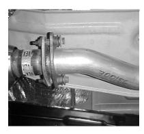
LAY OUT THE GIBSON EXHAUST SO IT LOOKS LIKE THE PICTURE AND COMPARE THE PART NUMBERS TO THE MANUAL TO MAKE SURE YOU HAVE THE CORRECT PART NUMBERS. THEN REMOVE THE FACTORY EXHAUST. FOR AN EASIER REMOVAL OF THE EXHAUST CUT JUST BEHIND THE MUFFLER ON THE TAIL PIPE. THEN UN-BOLT THE FACTORY FLANGE IN FRONT OF THE STOCK MUFFLER NOTE: **LEAVE ALL RUBBER GROMMETS IN PLACE. DO NOT DISGUARD HARDWARE** YOU WILL RE-USE IT.
