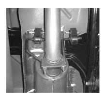
INSTALL HANGER #G ON THE OUTLET OF THE MUFFLER. DO NOT TIGHTEN.
