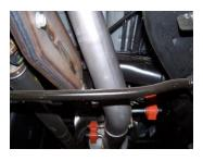
**7.** Install the over axle tailpipe #C into the extension pipe  $1\frac{1}{2}-2^{"}$ . Use clamp #E to secure. Do not tighten. Insert welded hanger into the rubber grommet.
