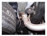
**3.** For easier removal of the stock exit pipe, remove rear hanger from the frame. Then remove exit pipe and re-install stock rear hanger.
