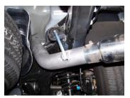
**8.** Install the exit pipe #D on the tailpipe. Secure together with clamp #E. Do not tighten. Roll the exit pipe until it is at the correct angle for your truck. Insert the welded hanger into rubber grommet.
