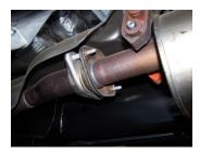
**2.** Remove the 2-bolt flange in front of your stock muffler. Also remove exit pipe from the clamp at the rear. Leave all rubber grommets in place. Use WD-40 to aid in removal of exhaust and hangers.
