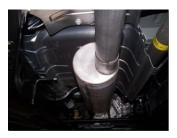
**3.** Install muffler #B onto head pipe 1½"-2" with the louvers facing towards the converter. Muffler inlet is looking into louvers. Use a jack stand to support the muffler. Outlet should be at the 4 o'clock position. Use clamp #F to secure the muffler to the headpipe. DO NOT TIGHTEN.
