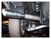
**5** Next, install the exit pipe #D to tailpipe. Use clamp #F to secure. DO NOT TIGHTEN. Insert welded hanger into rubber grommet.
