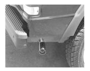
INSTALL THE STAINLESS STEEL TIP. USE ANY ALUMINUM OR STAINLESS STEEL CLEANER TO POLISH THE TIP. NOW TIGHTEN ALL CLAMPS, HANGERS, AND BOLTS.
