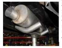
**INSTALL MUFFLER #C ONTO** TAILPIPE 1-1/2" TO 2" WITH INLET TOWARDS THE MOTOR. USE CLAMP #G TO SECURE THE TAILPIPE AND THE MUFFLER, DO NOT TIGHTEN. MUFFLER INLET SHOULD BE AT 9 O'CLOCK POSITION.
