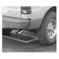
ROTATE TAILPIPE UNTIL YOU HAVE A MINIMUM OF 1" FROM ALL PIPES, RUBBER BRAKE LINES, TIRES, SWAY BAR, SHOCKS, ETC. THEN TIGHTEN ALL CLAMPS AND HANGERS. REINSTALL THE REAR SHOCK MOUNT. INSTALL YOUR STAINLESS STEEL TIP TO YOUR DESIRED LOOK. USE ANY ALUMINUM OR STAINLESS STEEL CLEANER TO POLISH YOUR TIP.
