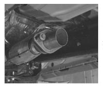
INSTALL FLANGE #G ONTO HEADPIPE #A. ATTACH TO FACORY FLANGE RE-USEING FACTORY BOLTS TO INSTALL IT. SNUG UP THESE BOLTS.
