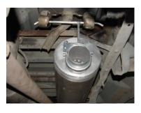
INSTALL MUFFLER #B ONTO HEADPIPE #A 1-1/2" TO 2". USE A JACKSTAND TO SUPPORT MUFFLER. SECURE MUFFLER TO HEADPIPE WITH CLAMP #I. DO NOT TIGHTEN. INSTALL HANGER #G ONTO OUTLET OF MUFFLER AND INSERT HANGERS INTO RUBBER GROMMETS. MUFFLER INLET IS LOOKING INTO THE LOUVERS.
