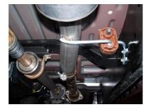
INSTALL HEADPIPE # A INTO STOCK PIPE. THE END OF THE PIPE SHOULD BE AT THE 12 O'CLOCK POSITION,. INSERT WELDED HANGERS INTO RUBBER GROMMET. ATTACH WITH FACTORY CLAMP. DO NOT TIGHTEN.
