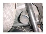
**6.** Install the over axle tailpipe # C into the muffler 1-1/2" to 2". Secure to the muffler using clamp # G Do not tighten.
