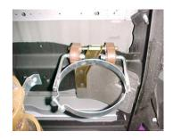
Install band clamp # F into rubber grommets located just above the axle. Do not tighten. And attach with bolt kit # I.
