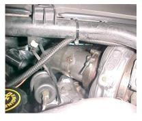
REMOVE THE REMAINING STOCK DOWN PIPE BY UNCLAMPING IT FROM THE TURBO HOUSING. USE A 11MM SOCKET OR WRENCH TO REMOVE YOUR STOCK PIPE THROUGH THE BOTTOM. DO NOT DISGARD THE STOCK CLAMP YOU WILL NEED TO RE-USE IT.
