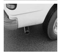
**INSTALL THE STAINLESS** STEEL TIP. USE ANY ALUMINUM OR STAINLESS STEEL CLEANER TO POLISH TIP. NOW TIGHTEN ALL CLAMPS, BOLTS AND HANGERS.
