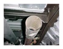
Install head pipe # A on to your new front pipe and secure with clamp # I Do not tighten.
