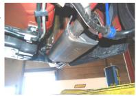
4. Now do the same procedure for the driver side tailpipes. Use clamp # C to secure the tailpipe to the muffler and stock clamp to secure it to the stock h-pipe.
