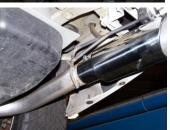
7. Install passenger side exit pipe #F onto tailpipe use clamp #I to secure pipes together. Insert welded hanger into rubber grommet. Do not tighten.
