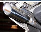
**8.** Install drivers side exit pipe #G. Use clamp #I to secure to the tailpipes together. Insert welded hanger into rubber grommets. Do not tighten.
