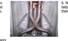
7. Now firmly tighten all bolts and clamps. Inspect all fasteners after 25-50 miles of operation and re-tighten as necessary.
