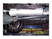
INSTALL MUFFLER #B ONTO HEAD PIPE 1-1/2" TO 2" WITH THE LOUVERS FACING TOWARDS THE CONVERTER. MUFFLER OUTLET SHOULD BE POSTIONED AT 12:00. USE A JACK STAND TO SUPPORT THE MUFFLER. USE CLAMP #E TO SECURE THE MUFFLER TO THE HEAD PIPE. DO NOT TIGHTEN. MUFFLER INLET IS LOOKING INTO THE LOUVERS.
