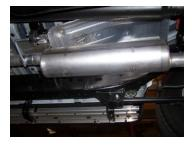
Install muffler #B onto head pipe #A 1-1/2" to 2" with the louvers facing towards the converter. Use a jack stand to support the muffler. Use clamp #F to secure the head pipe. Outlet of muffler will be at the 6 o'clock position. DO NOT TIGHTEN. Muffler inlet is looking into the louvers.
