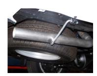
Install the exit pipe #D on the tailpipe. Secure together with clamp #F. DO NOT TIGHTEN. Roll the exit pipe until it is at the correct angle for your truck. Insert welded hanger into rubber grommet.
