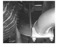
SLIP OVERAXLE PIPE #C INTO THE OUTLET OF THE MUFFLER NO MORE THEN 2" AND NO LESS THEN 1 ½". USE HANGER # G TO HANG THE OVERAXLE PIPE. THE SPARE TIRE MAY NEED TO BE LOSENED AND PUSHED TO THE REAR OF THE TRUCK TO GAIN CLEARANCE FOR INSTALLATION OF OVERAXLE PIPE. INSTALL THE EXIT PIPE #D AND CLAMP TO HANGER #G.
