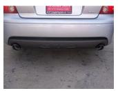
**5.** When you have everything in place, firmly tighten all bolts and clamps down securely. Use stainless steel cleaner and a Scotch Brite pad weekly to prevent tip from discoloration.
