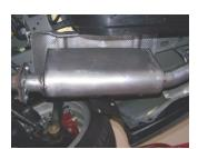
**2.** Unbolt factory muffler from flange located in front of muffler and remove. Repeat for other side.
