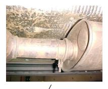
/ UNCLAMP FOR EASIER REMOVAL OF THE FACTORY EXHAUST.
