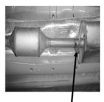
FOR EASIER REMOVAL OF THE FACTORY EXHAUST. CUT THE TAILPIPE BEHIND THE MUFFLER. THEN REMOVE THE FACTORY MUFFLER AT THE CLAMP IN FRONT OF THE MUFFLER. USE A JACK STAND TO SUPPORT THE CONVERTER ONCE EXHAUST IS REMOVED. NOTE LEAVE ALL FACTORY RUBBER GROMMETS IN PLACE
