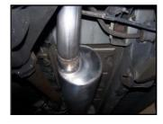
**3.** Install the Gibson muffler in the same position as the stock muffler and clamp to stock pipe with clamp #D. Muffler may angle down at back. Inlet of muffler is looking into the louvers. DO NOT TIGHTEN.
