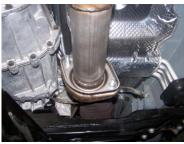
Install head pipe # A onto your existing stock flange and secure with bolt kit #F. DO NOT TIGHTEN.
