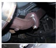
floor so it looks like the drawing and compare parts with manual. Remove the stock exhaust from the 3 bolt flange just behind the muffler, then remove the back section, then the remaining stock exhaust from the 2 bolt flange in front of the muffler. Leave all rubber grommets in place. Use WD-40 to aid in removal of hangers.
