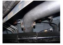
Install extension pipe #C into the muffler 1½-2". Insert welded hanger into rubber grommet. Secure the muffler using clamp #E. DO NOT TIGHTEN.
