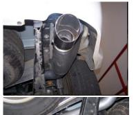
Install the over axle tail pipe w/welded resonator onto extension pipe, insert welded hangers into grommets and use clamp #E to secure pipes together. DO NOT TIGHTEN.
