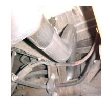
INSTALL TAILPIPE # B INTO MUFFLER 1 ½" – 2". INSERT WELDED HANGER INTO RUBBER GROMMET, ROTATE PIPE SO YOU HAVE PROPER CLEARANCE. USE CLAMP # D TO SECURE PIPE TO MUFFLER. DO NOT TIGHTEN.
