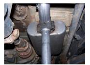
4. Install muffler #B onto headpipe #A 1.5-2" with the louvers facing towards the converter. Use a jack stand to support the muffler. Use clamp #D to secure the muffler to the headpipe. Do not tighten. Muffler inlet is looking into the louvers.
