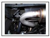
**3.** Install head pipe #A onto your existing stock front pipe and attach with clamp #E. Insert welded hanger into rubber grommet. Do not tighten.
