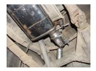
Next install front tailpipe #B into muffler 1 ½ to 2". The shorter side goes into the muffler. Use clamp # F to secure pipe to muffler. Slide welded hangers into rubber grommets.
