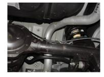
INSTALL TAILPIPE #D INTO MUFFLER 1-1/2" TO 2". INSERT WELDED HANGER INTO RUBBER GROMMET. USE CLAMP #F TO SECURE TAILPIPE TO MUFFLER. ROTATE THE TAILPIPE UNTIL IT IS LEVEL.
