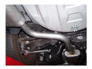
4. Install driver side tailpipe/muffler assembly #B. Insert all welded hangers into rubber grommets. Secure tailpipes with clamp #D. Do not tighten.
