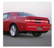
7. Re Install Stock Tips. Use stainless steel cleaner and a Scotch Brite pad weekly to prevent tips from discoloration. Inspect all fasteners after 25-50 miles of operation and retighten as necessary.
