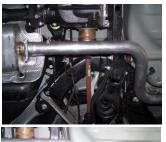
3.Next, install tailpipe assembly #B onto headpipe assembly, secure with clamp #C. DO NOT TIGHTEN.
