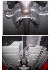
2. Install headpipe assembly #A onto stock Y-pipe. Secure pipe with clamp #C. DO NOT TIGHTEN. Use jackstand to support muffler.
