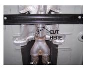
1. To remove the stock exhaust, First remove the crossmember. Measure 3" back from weld on the Y-pipe and cut. Remove all hangers from rubber grommets. Use WD-40 to aid in the removal of the hangers. Then carefully remove the stock exhaust.
