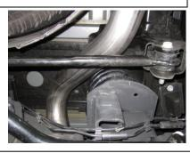
4. Install over axle pipe Item # B into the muffler outlet 1.5" to 2". Slip the hangers into the rubber grommets and keep tailpipe loose use clamp #c to secure together.
