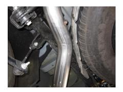
6. With proper clearance from spare tire install the exhaust tip onto the tailpipe. The system was designed to have the tip 1" below the quarter panel of the vehicle. With the tip in your desired position begin to tighten down all clamp connections from the front head pipe back.
