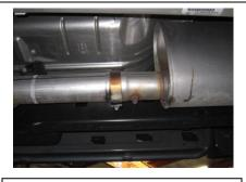
1.Remove from the first clamp located in front of the muffler.
