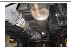
3. Install muffler assembly #A onto factory pipe insert hangers into rubber grommets use clamp #c to secure together do not tighten.
