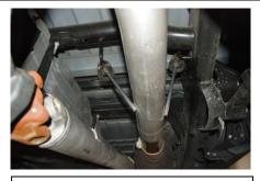
3. Install the over axle pipe Item # B onto the Gibson head pipe. Install the hangers into the factory rubber grommets. Adjust to desired position and to not tighten.
