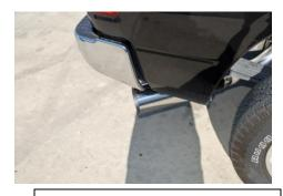
7. The system was designed to have the tip 1" below the quarter panel of the vehicle. With the tip in your desired position begin to tighten down all clamp connections from the front head pipe back. Clean tip before starting vehicle.
