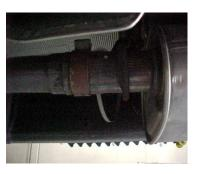
Lay out the exhaust on the floor so it looks like the drawing and compare parts with manual. To remove the stock exhaust remove it from the clamp in front of the muffler, remove ground strap, do not disguard hardware you will re-use it. You may need to heat it up for easier removal. Leave all rubber grommets in place. Use WD-40 to aid in removal of exhaust and hangers.
