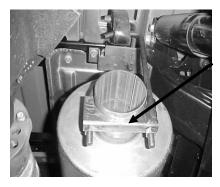
INSTALL REAR MUFFLER HANGER #G TO OUTLET OF MUFFLER. INSERT WELDED HANGER INTO RUBBER GROMMET. THE VERTICAL BAR ON THE HANGER IS ON THE PASSENGER SIDE. DO NOT TIGHTEN.
