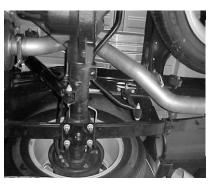
INSTALL OVERAXLE TAILPIPE #B AND CONNECT TO THE MUFFLER USING HANGER # G. INSERT WELDED HANGER INTO RUBBER GROMMETS.
