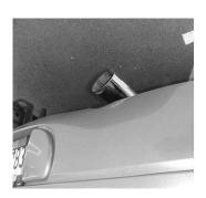
INSTALL THE STAINLESS STEEL TIP. USE ANY ALUMINUM OR STAINLESS STEEL CLEANER TO POLISH YOUR STAINLESS STEEL TIP. FIRMLY TIGHTEN ALL CLAMPS AND HANGERS.
