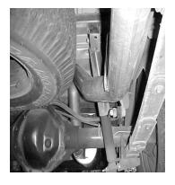
INSTALL OVERAXLE TAILPIPE #C AND CONNECT IT TO THE MUFFLER AND CLAMP DOWN USING HANGER #D. INSERT WELDED HANGER INTO RUBBER GROMMET. ROLL THE TAILPIPE UNTIL YOU FIND THE CORRECT ANGLE. THE SPARE TIRE ON SOME VEHICLES MAY NEED TO BE LOOSENED AND PUSHED TO THE DRIVER SIDE FOR CLEARANCE PURPOSES.
