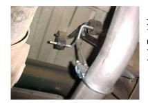
INSTALL THE OVERAXLE TAILPIPE #C TO THE MUFFLER. USE CLAMP #E TO SECURE PIPE TO MUFFLER. BUT DO NOT TIGHTEN.
